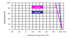
Derating Output Current Versus Ambient Temperature and Airflow  $$V_{\text{in}}$=V_{\text{in nom}}$$
