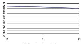
Efficiency Versus Input Voltage Full Load
