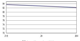
Efficiency Versus Input Voltage Full Load
