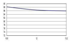
Efficiency Versus Input Voltage Full Load
