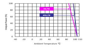
Derating Output Current Versus Ambient Temperature and Airflow  $\label{eq:Vin} V_{\text{in nom}}$
