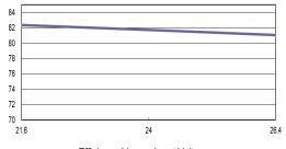
Efficiency Versus Input Voltage Full Load
