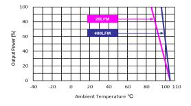
Derating Output Current Versus Ambient Temperature and Airflow  $$V_{\text{in}}$=V_{\text{in nom}}$$
