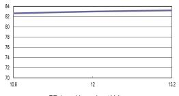
Efficiency Versus Input Voltage Full Load
