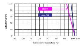
Derating Output Current Versus Ambient Temperature and Airflow  $\label{eq:Vin} V_{\text{in nom}}$
