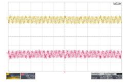
Typical Output Ripple and Noise Vin=Vin nom ; Full Load
