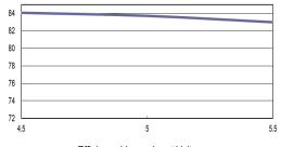
Efficiency Versus Input Voltage Full Load
