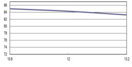
Efficiency Versus Input Voltage Full Load
