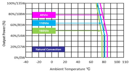
Derating Output Power Versus Ambient Temperature (with 3U iron back-plate (Dimension 482X133.5X1.6mm))
