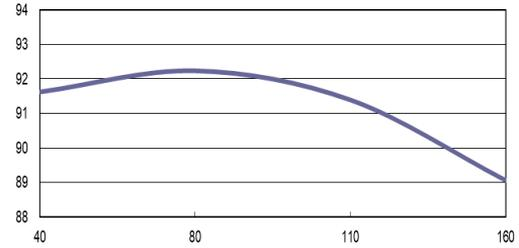
Efficiency Versus Input Voltage
