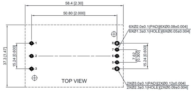
**Recommended Pad Layout ( $\pm$ Vout pin  $\varnothing$ 1.5mm)**
