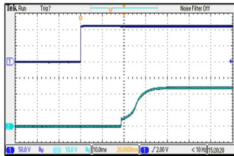
ON/OFF Voltage Start-Up and Output Rise Characteristic
