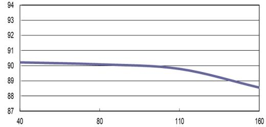
Efficiency Versus Input Voltage
