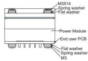
**PCB Installation of End Users ( $\pm V_{out}$  pin  $\varnothing 1.5\text{mm}$ )**
