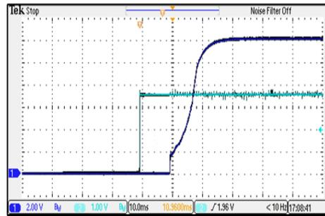
ON/OFF Voltage Start-Up and Output Rise Characteristic
