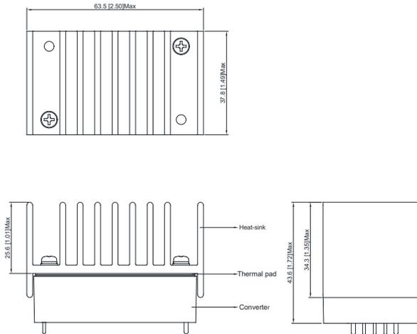
**PCB Installation of End Users ( $\pm V_{out}$  pin  $\varnothing 2.0\text{mm}$ )**
