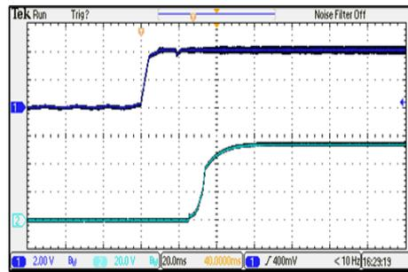
ON/OFF Voltage Start-Up and Output Rise Characteristic
