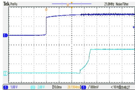
ON/OFF Voltage Start-Up and Output Rise Characteristic
