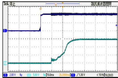
ON/OFF Voltage Start-Up and Output Rise Characteristic
