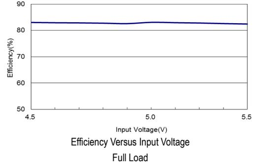
Efficiency Versus Input Voltage Full Load
