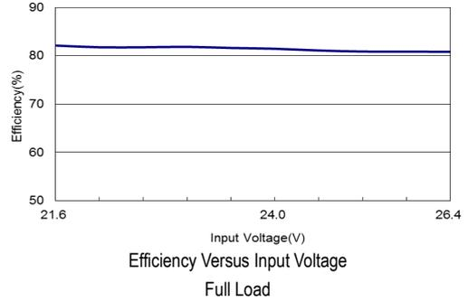
Efficiency Versus Input Voltage Full Load
