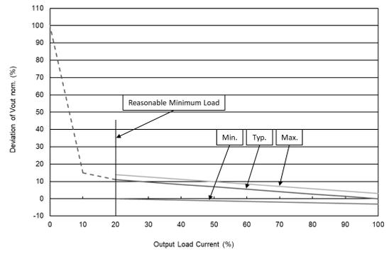
**MBU135 & MBU131 Output Voltage VS Output Load Current**
