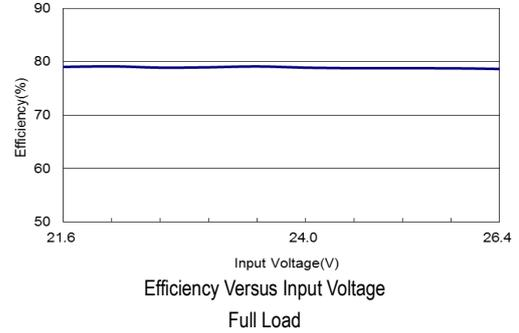
Efficiency Versus Input Voltage Full Load
