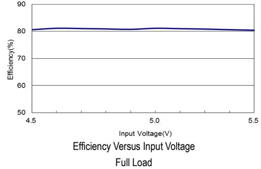
Efficiency Versus Input Voltage
