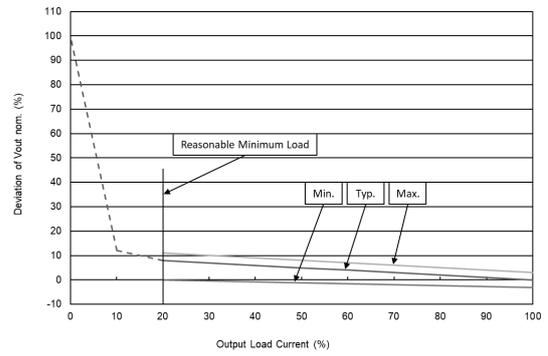
**MBU111 Output Voltage VS Output Load Current**
