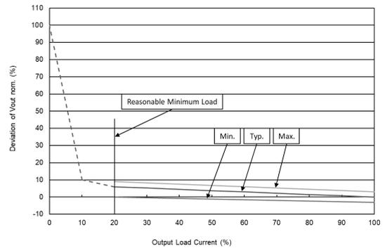
**MBU103 Output Voltage VS Output Load Current**
